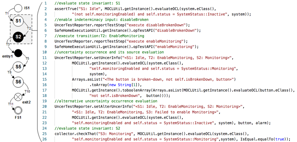
Fig. 4. An example representing the logic of an abstract and an executable test cases (partial) generated by UncerTest
