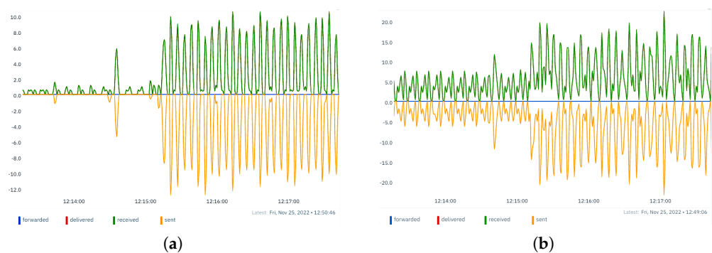
Figure 10. The variation in IPV4 Network Packets by ML model (a) Jetson, (b) Raspberry Pi (y → packets & x → time).
