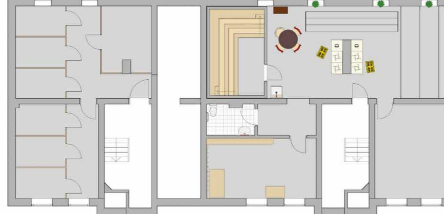
storage units for the residents the two-room apartments on the second and third floor has a unit each (the six along the left wall) the large unit is shared between the residents of the collective on the top floor
